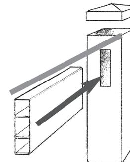
2. **Build Out First Short Side** – Continue assembly of the post and rail using the method described above. The guide string between the corner stakes is used to keep the line straight as you build to the next corner.
