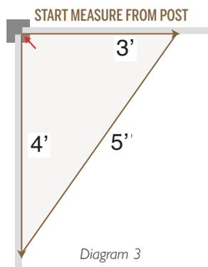
8. **Layout Second Long Side** – Tie a string between the two stakes to layout your second long side. You may need to adjust one of the short side stakes to get the arena square.
